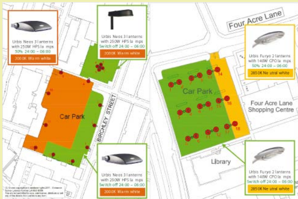
New LED lighting controlled through CMS – 66% energy saving. St. Helens. (TCS 5.2 5.3)
