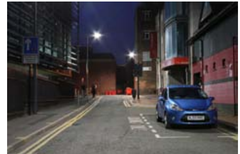
New LED as part of central St. Helens regeneration scheme - 24% energy saving. (TCS 4.2)
