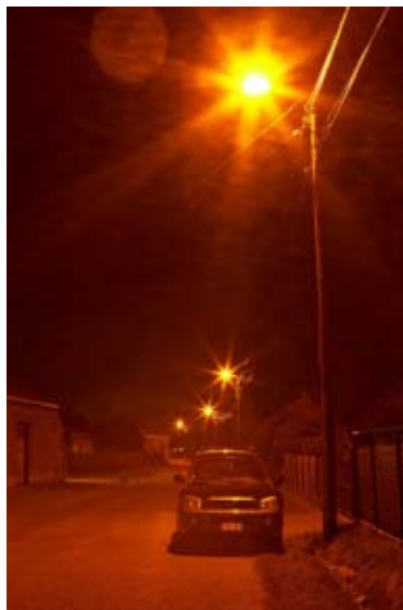
New white light Cosmopolis 60W lamp providing high-quality colour rendition and illumination compared to SON light source in surrounding residential areas. St. Helens. (TCS 7.1)
