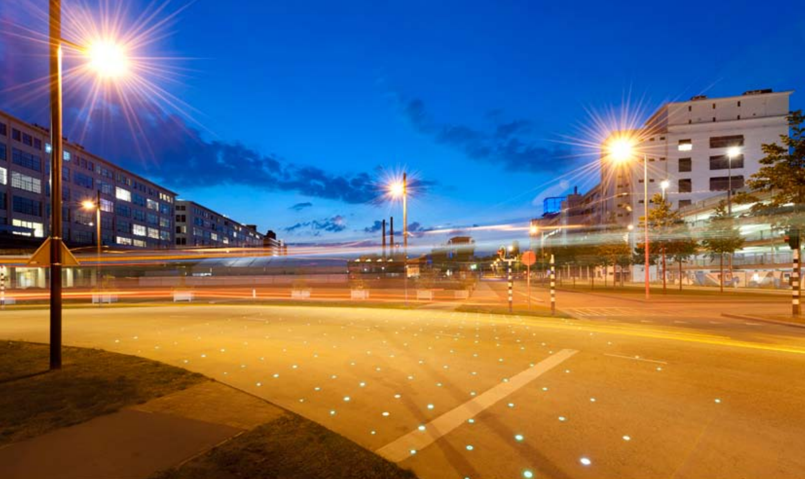
HOV bus lane crossing is RGB LED's in the ground react to sensors and pedestrians crossing. To replace traditional crossing lights. Strijp-S, Eindhoven. (TCS 6.7)
